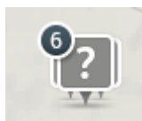
Figure 6-4: Wind power plant icon – several wind power plants. In this example, one or more wind turbines are not in operation. In case of more wind turbines with events, the icon for the most severe state is displayed (for an overview of severity ranking - see Table 7-2: Wind turbine status icons).
